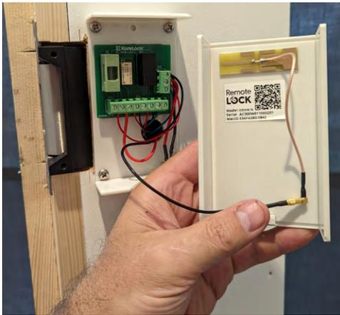
**21. Connect the Wi-Fi antenna lead to the connector on the rear of the white enclosure cover.**
