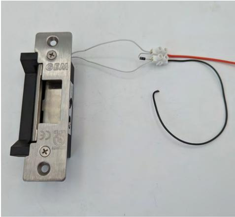
**16. Remove the electric strike and fit the diode as per the wiring diagram.** The diode has a white ring on one side. This should connect to the +12V wire. The diode protects the electronics from unexpected power surges. Wrap some electrical insulation tape around the connector (*not shown here*).
