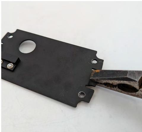
**11. If fitting the gasket, use pliers to carefully bend the top tap up slightly.** This makes aligning the keypad easier. There is no need to do this if fitting the rainshield.
