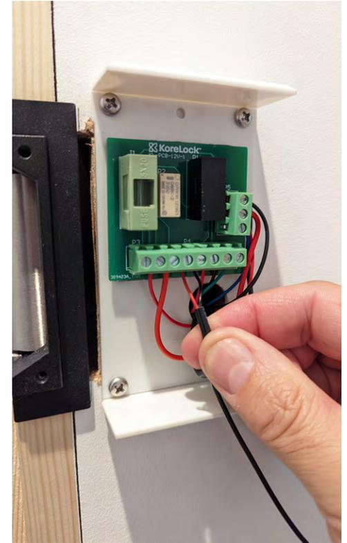
**20. The black 2 core cable from the keypad connects to either SEC terminals.** This is a safety feature, if someone removes the keypad from the backplate then the power will switch off until the keypad is returned to the backplate.
