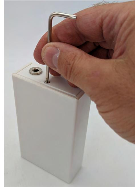
**3. Using the included security wrench, remove the T10 screw from the underside of the white enclosure.** The cover unclips from the top side by slightly pushing out the cover sides so that it can slide off.
