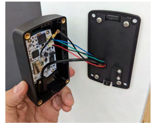
**13. Feed the 4 cables through the hole, making sure to pull them through the hole in the enclosure.** Do not pull tight, you should leave some slack cable within the keypad body.
