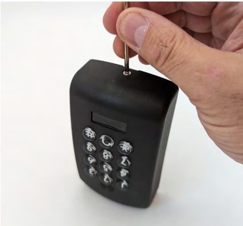
**7. Remove the T10 security screw from the keypad using the included wrench.**
