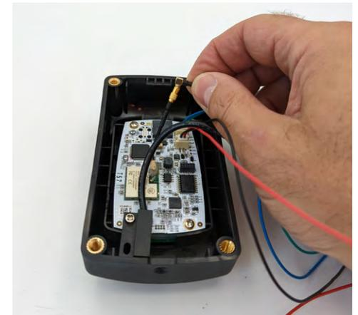
**10. Plug in the red/black and blue/green cables as per the wiring diagram. Also connect the Wi-Fi antenna lead. You should have 4 cables.**
