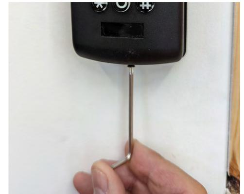
**15. Secure the keypad in place with the T10 security screw.**
