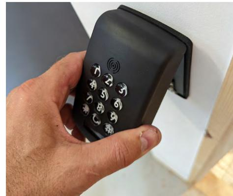
**14. Hold the keypad at an angle and insert into the backplate.** It must be perfectly aligned. If it will not locate, try bending the tab a 'little' more, but not too much as it could snap.
