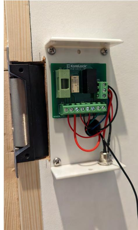
**19. Connect the 4 cables as per the wiring diagram.**
